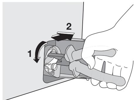
7. Remove foreign bodies and fluff from the pump seat and from the pump impeller.
