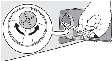
9. Replace the filter into the pump by inserting it correctly into the special guides. Screw the pump cover firmly by turning it clockwise.
