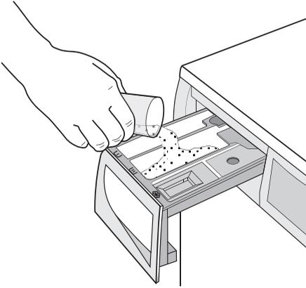
If required, pour fabric softener into the compartment marked
