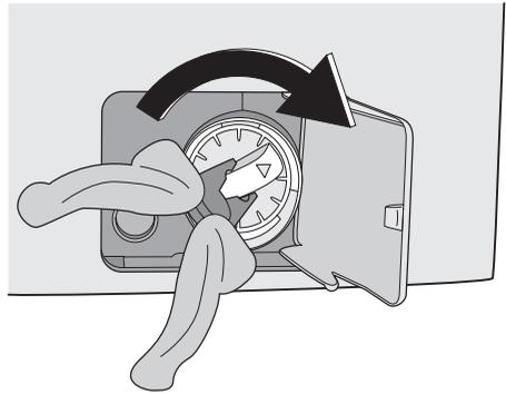
10. Replace the emergency emptying cap into the filter cover and fix it firmly.
