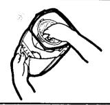
When dust has been settled in the dust container, reinstall the expander to the cloth filter by turning it clockwise. Remove the cloth filter from the dust container.
