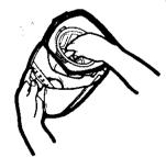
Reattach the filter unit to the dust container.
