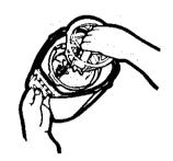
Pull the expander upward by turning it counterclockwise. Shake the expander to the right and left about 20 times.
