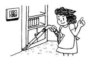
For a slight cleaning job, apply curved wand of hose directly without any cleaning tools and extension wands.
