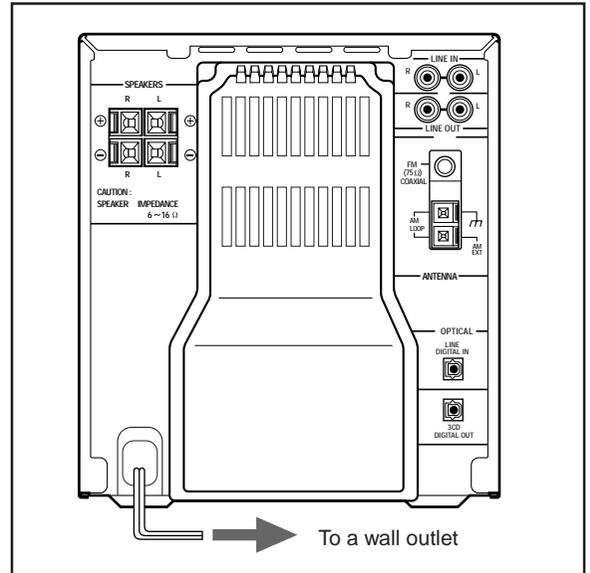
Connect between the optical digital input terminal on the other component and the 3CD DIGITAL OUT terminal.
