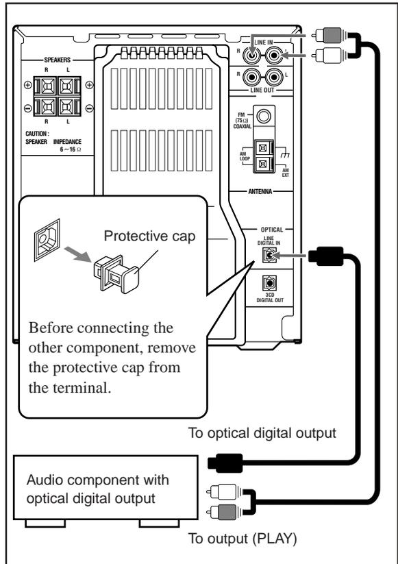
By using an optical digital cord (not supplied) and an audio cord (not supplied), connect:
