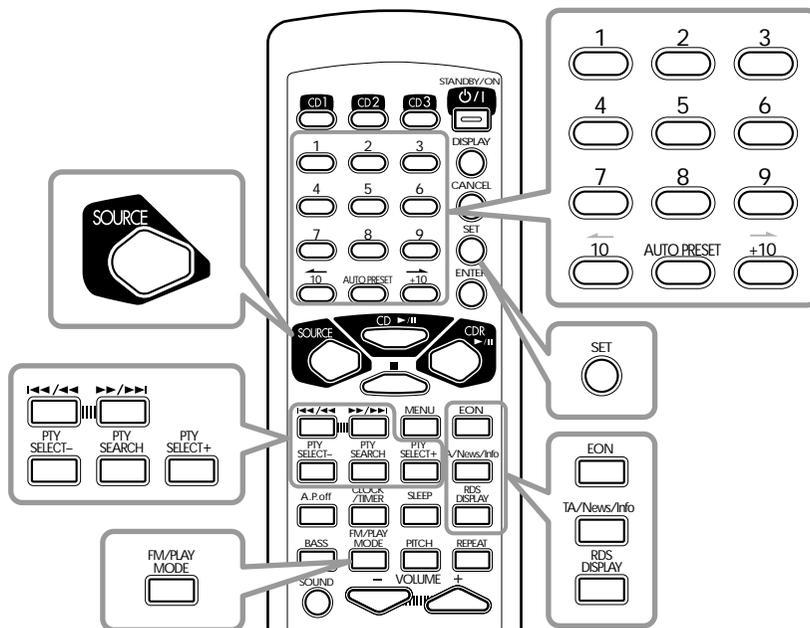
You cannot use the buttons on the front panel to operate the RDS functions. Use only buttons printed in orange on the remote control.
