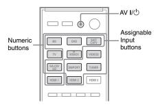
1 While holding down the input button of which you want to change the assignment, hold down AV I/().
