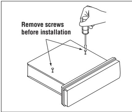
**Note:** If this unit is to be installed in a boat or a spa, you should use the two pieces of plastic film (30 mm X 20 mm) supplied to seal the two holes after removing the screws.
