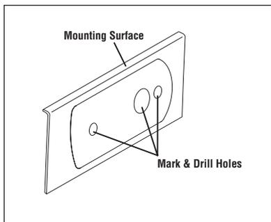
2. Remove the foam adhesive backer and drill two 3/8" and one 5/8" mounting holes in the marked positions.
