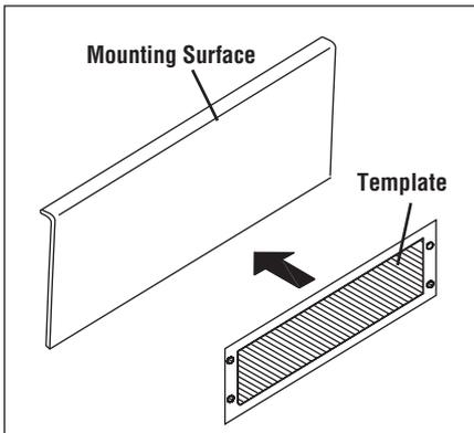
2. Cut and remove the hatching area on the template. Then drill four 1/8" mounting holes in the exact position according to the mounting paper.
