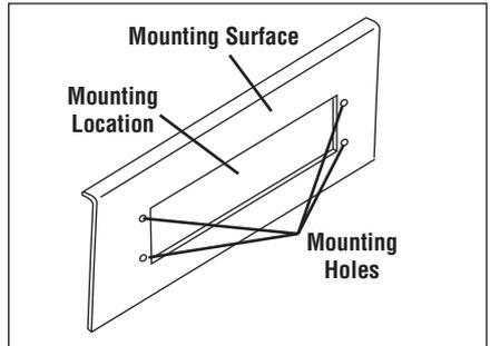
3. Use the glue paper to stick the two mounting brackets to the back of the mounting surface. The screw holes of the brackets must respectively aim at the mounting holes in order to fix the unit to the mounting surface.
