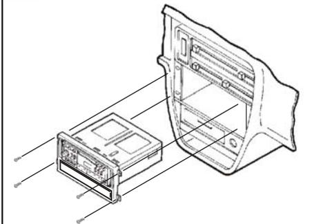
Re-connect the battery terminal and test the unit for proper operation. Mount the head unit/kit assembly to the sub-dash with (4) screws previously removed.
