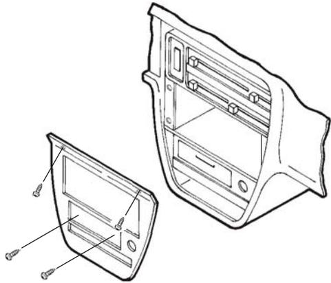
Disconnect the negative battery terminal to prevent an accidental short circuit. Remove the ashtray and (2) Phillips screws exposed. Remove (2) Phillips screws above the radio opening. Unclip the radio trim bezel and disconnect the cigarette lighter wiring. Remove (2) screws securing each side of the factory head unit and (1) screw from the rear support. Slide the unit out and disconnect the wiring.
