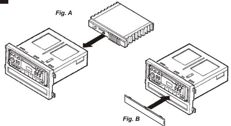
**IF AN EQUALIZER WILL BE INCLUDED:** Slide the aftermarket equalizer into the back of the *Radio Housing*. Using the hardware included with the equalizer, mount the unit to the kit. (see Fig. A)
