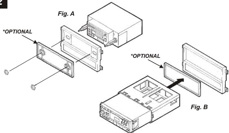
**2-SHAFT HEAD UNITS:** Slide the aftermarket head unit into the kit and secure with shaft nuts. (see Fig. A)
