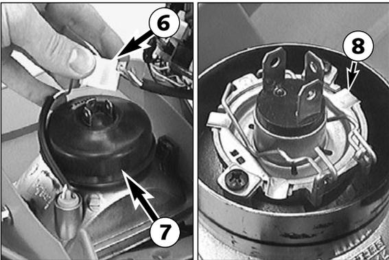
Hook in the retaining bracket, mount the rubber cap and connect the plug to the bulb.
