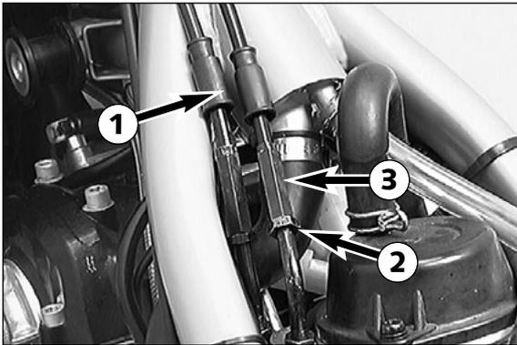
If a correction is necessary, start by removing the tank. Slide back the protection cover ①. To set the backlash, loosen the counter nut ② and turn the adjusting screw ③ accordingly. Then, fasten the counter nut and slide the protection cover back on.
