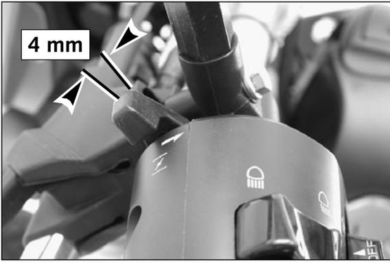
**Checking and adjusting the choke cable play \***
