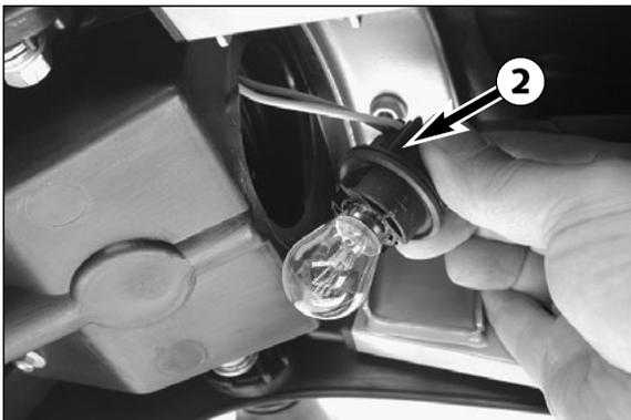
Turn the lamp socket ② approximately 30° counterclockwise and pull it out of the tail light housing.
