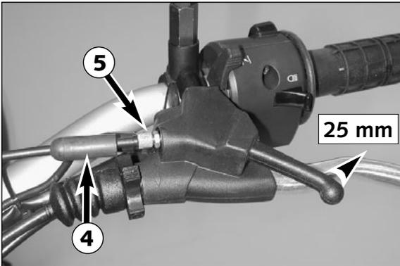
**Checking the adjustment of the hand decompression cable\***
