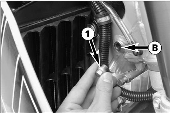
Fill 0.6 liters of engine oil into the can and remove the plug 1 next to the steering head. Introduce the plastic hose into the vent hole B, (see page 30) and fill 0.6 liters of engine oil into the frame's front tube. Remove plastic hose, start engine, and let it idle (approx. 20 seconds) until oil escapes at the hole B. As soon as oil starts to escape, turn off the engine, and mount the plug together with the gasket.
