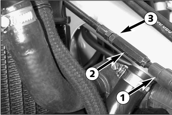
Push the choke lever all the way to the front and slide the protecting cap **1** from the adjusting part **2**. Loosen the lock nut **3** and correct the play by turning the adjusting part. Tighten lock nut and slide protecting cap back on. Mount the tank and seat.
