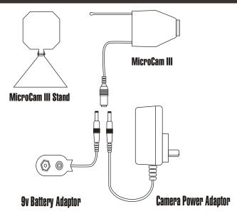
IMPORTANT: Due to the power consumption requirements of this product, we highly recommend the use of a 9 volt battery only for short term portable use.
