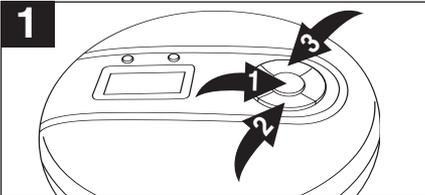
With a CD inserted, press the PLAY/PAUSE (▶||)/POWER ON button ❶ to turn the unit on and press the STOP (■)/POWER OFF button ❷ to stop auto playback. Press the MODE button ❸ four times; the RAND indicator will appear in the display.
