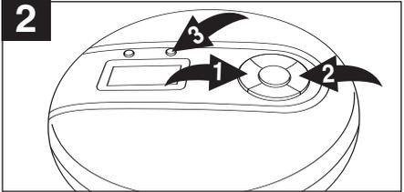
Select the first track to be played back using the SKIP/SEARCH ◀① or ▶② button, then press the PROG button ③ again. Repeat this step to program additional tracks up to a maximum of 24 tracks.
