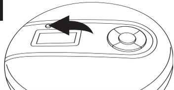
To turn the Anti-Shock System off, press the ESP button.
