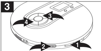
Adjust the VOLUME control ❶ and DBBS switch ❷ as desired. To **skip** forward or backward through the tracks on the disc, press the SKIP/SEARCH ◀❸ or ▶❹ button. To **search** forward or backward through the tracks on the disc, press and hold the SKIP/SEARCH ◀❸ or ▶❹ button.
