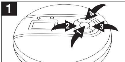
With a CD inserted, press the PLAY/PAUSE (▶||)/POWER ON button ❶ to turn the unit on, then select a track using the SKIP/SEARCH ◀❷ or ▶❸ button. Press the MODE button ❹ once; the Repeat 1 indicator
