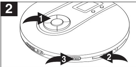
The unit will then play the same track over and over until the STOP (■)/POWER OFF button ❶ is pressed. Adjust the VOLUME control ❷ and DBBS switch ❸ as desired.
