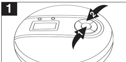
With a CD inserted, press the PLAY/PAUSE (▶||)/POWER ON button ❶ to turn the unit on. Press the MODE button ❷ twice; the Repeat All indicator
