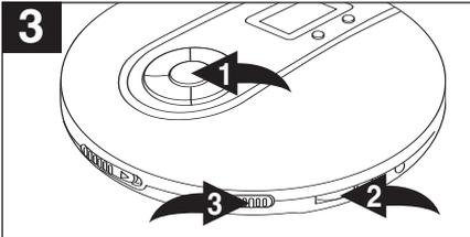
Press the PLAY/PAUSE (▶||)/POWER ON button ① to begin Programmed playback and adjust the VOLUME control ④ and DBBS switch ⑤ as desired.
