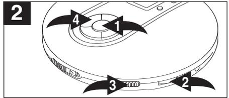
Press the PLAY/PAUSE (▶||)/POWER ON button ❶ to begin playback. The unit will play all the tracks in random order. Adjust the VOLUME control ❷ and DBBS switch ❸ as desired. When all the tracks have been played, the unit will stop. Press the STOP (■)/POWER OFF button ❹ to stop Random playback.
