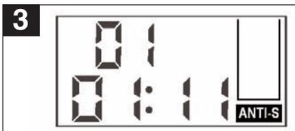
3 The Anti-Shock System will start automatically, the sound will mute for a moment and the display will show the Anti-Shock indicator with no bars in it.
