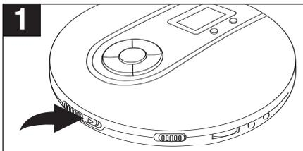
1 Open the CD compartment lid by sliding the CD OPEN switch to the right. Gently press a disc, label side up, onto the spindle until it locks in place. Close the CD compartment lid. Insert headphones into the PHONES jack.
