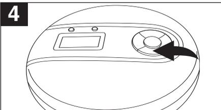
When the disc is through playing, it will stop. Press the STOP (■)/POWER OFF button to stop the disc before it is finished; the total number of tracks will appear. Press the STOP (■)/POWER OFF button again while in the stop mode to turn the unit off or wait approximately 60 seconds and the unit will automatically turn off.
