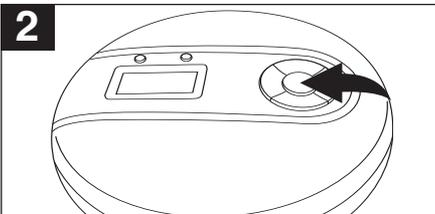
2 With a CD inserted, press the PLAY/PAUSE (▶||)/POWER ON button to turn the unit on.
