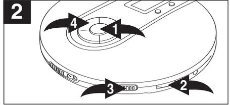
Press the PLAY/PAUSE (▶||)/POWER ON button ❶ to begin playback. The unit will play the first 10 seconds of each track. Adjust the VOLUME control ❷ and DBBS switch ❸ as desired. Press the STOP (■)/POWER OFF button ❹ to stop Intro playback.
