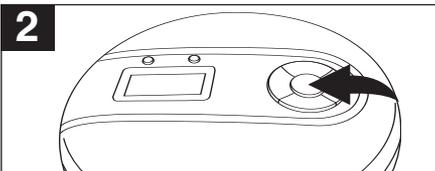
Press the PLAY/PAUSE (▶||)/POWER ON button to start playback. To pause **PLAYBACK**, press the PLAY/PAUSE (▶||)/POWER ON button again, the elapsed time will blink. Press once again to resume playback.
