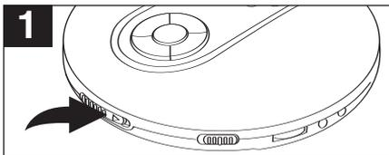
Open the CD compartment lid by sliding the CD OPEN switch to the right. Gently press a disc, label side up, onto the spindle until it locks in place. Close the CD compartment lid. Insert headphones into the PHONES jack.
