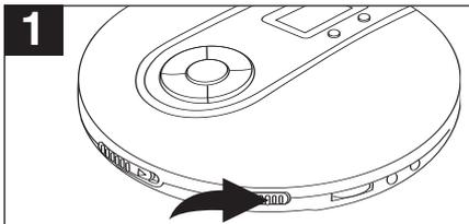
To emphasize the bass, slide the DBBS switch to the ON position. For normal bass, slide the DBBS switch to the OFF position.
