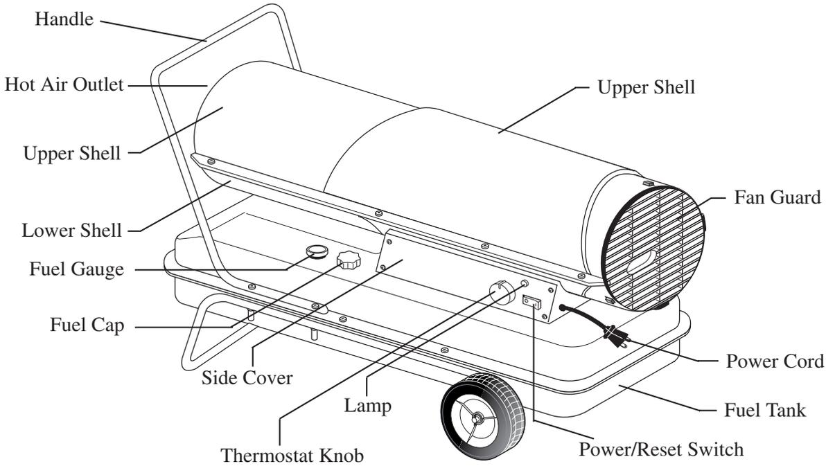
**Figure 2. RMC-KFA120T / RMC-KFA170T MODELS**
