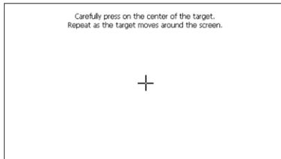
Tap the center of the cross with your finger. When the cross moves to another position, tap and hold the center of the new target. Repeat each time to complete the calibration process. When tapping the screen on the final step, the new settings will be stored and you are returned to the Display menu.
