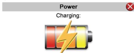
The Power menu displays the unit's battery status. The values are between 0% and 100%, where 0% means the battery power has run out completely, and 100% represents a full battery power. When the battery is being charged, the Battery Status will indicate "Charging".
