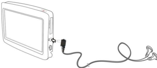
When earphones are connected, the speaker will automatically turn off.
