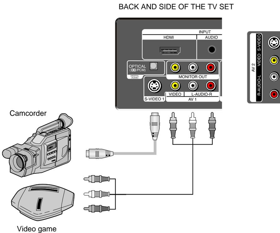
**Note:** If your AV device has both Video OUT terminal and S-Video OUT terminal, S-Video connection is recommended for better picture quality.
