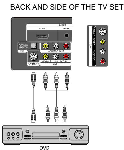
**Note:** If your AV device has both Video OUT terminal and S-Video OUT terminal, S-Video connection is recommended for better picture quality.
