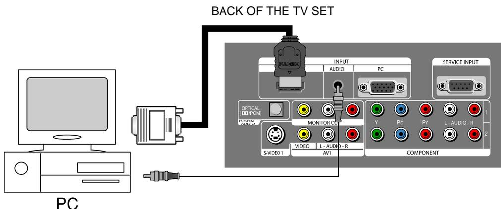
**Note:** If the graphic card of the PC only supports a DVI signal, you must connect the Audio cable like above the picture.
