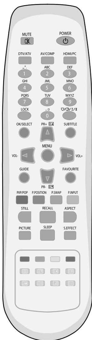
21. **RECALL** : Display the present modes (ATV/DTV, Video 1/2, Comp. 1/2, PC/HDMI) and Signal information for 4 seconds.
