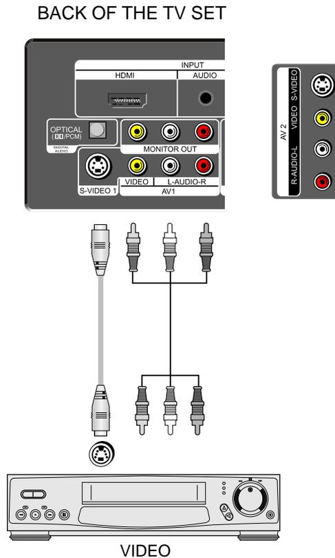
**Note:** If your AV device has both Video OUT terminal and S-Video OUT terminal, the S-Video connection is recommended for better picture quality.
