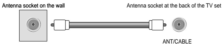
**When a feeder cable is used:** Plug the coaxial cable to the antenna socket, and fix it firmly by turning it to the right.
