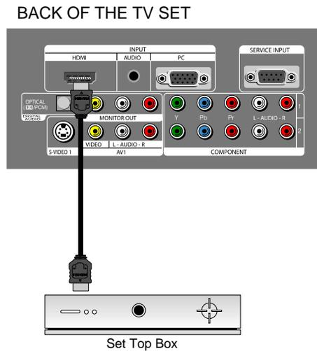
**Note:** When the Set Top Box output is DVI signal, then the Audio cable should be connected.
