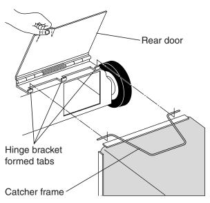
**ACAUTION:** Under normal usage, the catcher material is subject to deterioration and wear and should, therefore, be checked frequently for replacement. Any replacement catcher should be checked to ensure compliance with original manufacturer's specifications.
