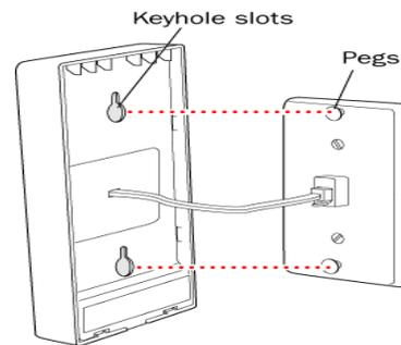
3. Connect the telephone cord to the phone jack located on the front of the mounted filter.
