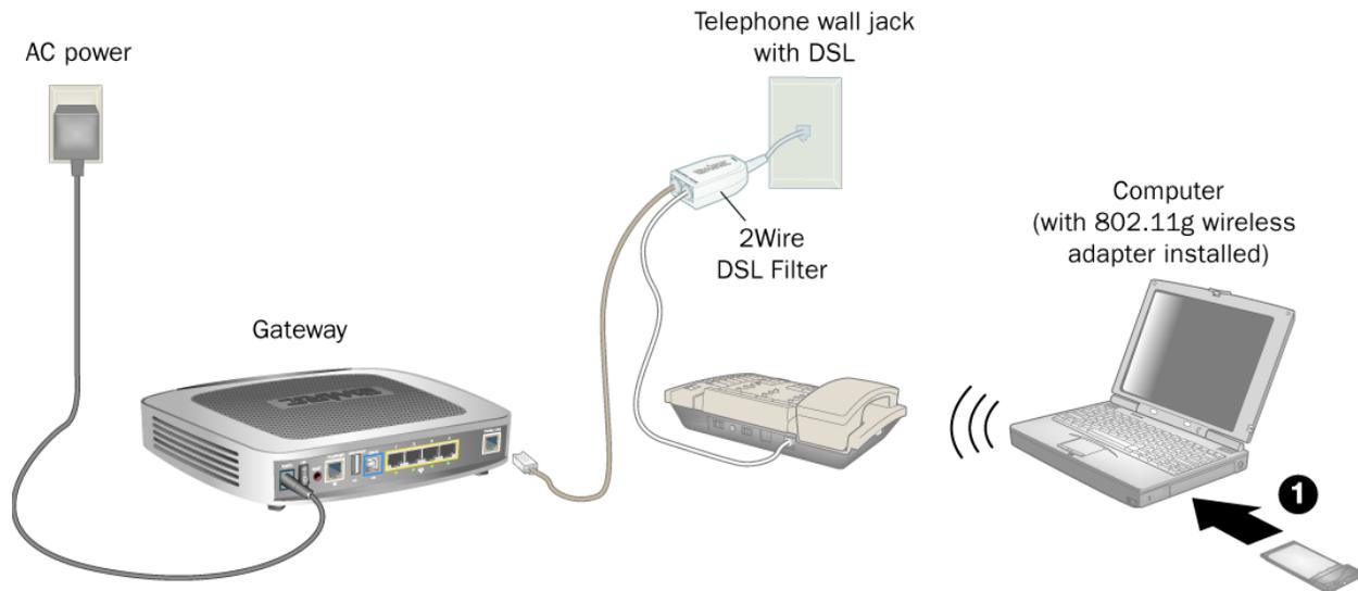
**Figure 6. Gateway Connected to Second Computer Via Wireless**
