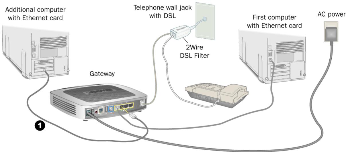
**Figure 4. Gateway Connected to Second Computer Via Ethernet**
