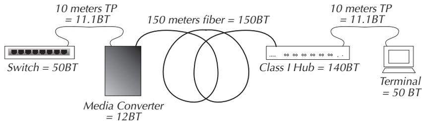
Since the total of the bit-times in this example is less than 512 (see chart below), the path is good.
