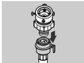
2. First, using a "+" type screw driver, loosen the four screws on the adaptor. Next, take the adaptor and turn part (b) following the arrow for gap about 5mm between them.
