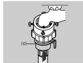
4. Connect the water supply hose to the adaptor. Pull down the part (c) of the water supply hose. When you release part (c) the hose is automatically connects to the adaptor making a 'click' sound.
