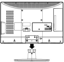
**4** Secure the wall mount bracket to the back of your TV using one M4 screws, as indicated in the illustration.
