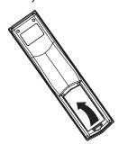
2 Insert two AAA batteries into the battery compartment. Make sure that you match the + and – symbols on the batteries with the + and – symbols in the battery compartment.
