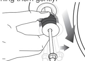
3. Fit the covers (supplied in the bag with the Operation Manual) into the holes on the rear panel. ("P")
