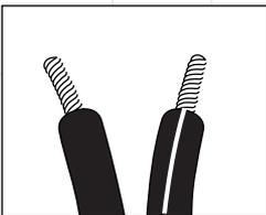
Separate and strip the ends of the speaker wire as shown. Speakers and electronics terminals have corresponding (+) and (-) terminals. Most manufacturers of speakers and electronics, including JBL, use red to denote the (+) terminal and black for the (-) terminal. The (+) lead of the speaker wire is noted with a stripe. It is important to connect all speakers identically: (+) on the speaker to (+) on the amplifier and (-) on the speaker to (-) on the amplifier. Wiring “out of
