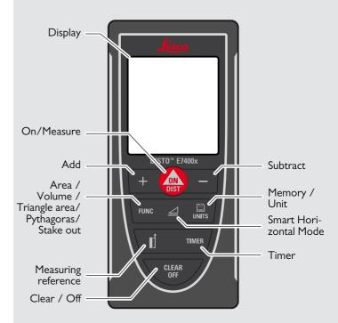
Instrument Set-up EN
