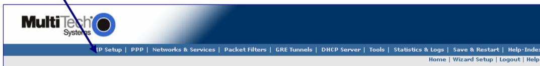
**IP Setup:** Sets up a General Configuration, HTTP, DDNS, SNTP, Static Routes, and Remote Configuration.
