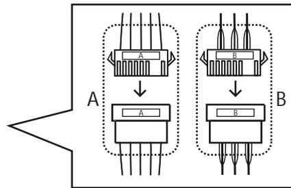
Following the labels (A to A & B to B) to plug the connectors.
