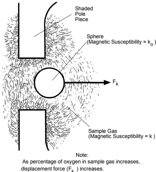
Figure 4-2. Spherical Body in Non-Uniform Magnetic Field
