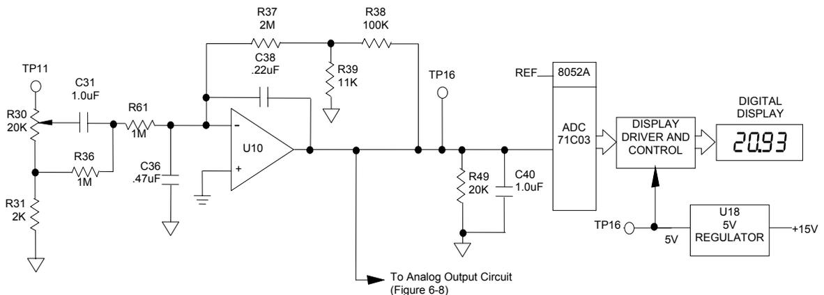
**Figure 5-7. Buffer, Anticipation, and Digital Output Circuits**
