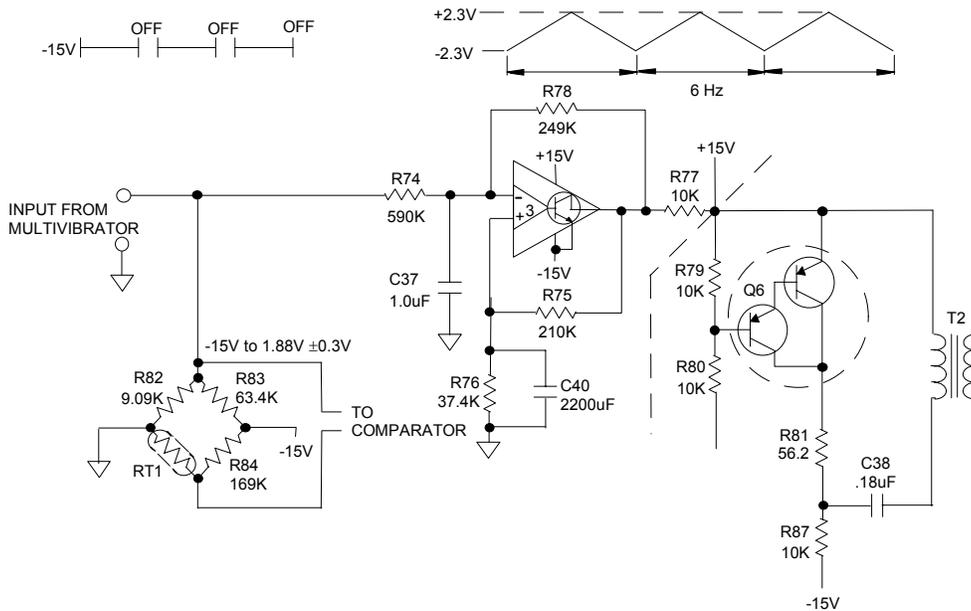
Figure 5-3. Ramp Generator Circuit
