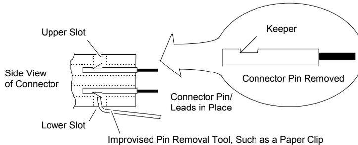
**Figure 6-2. Pin/Lead Removal**
