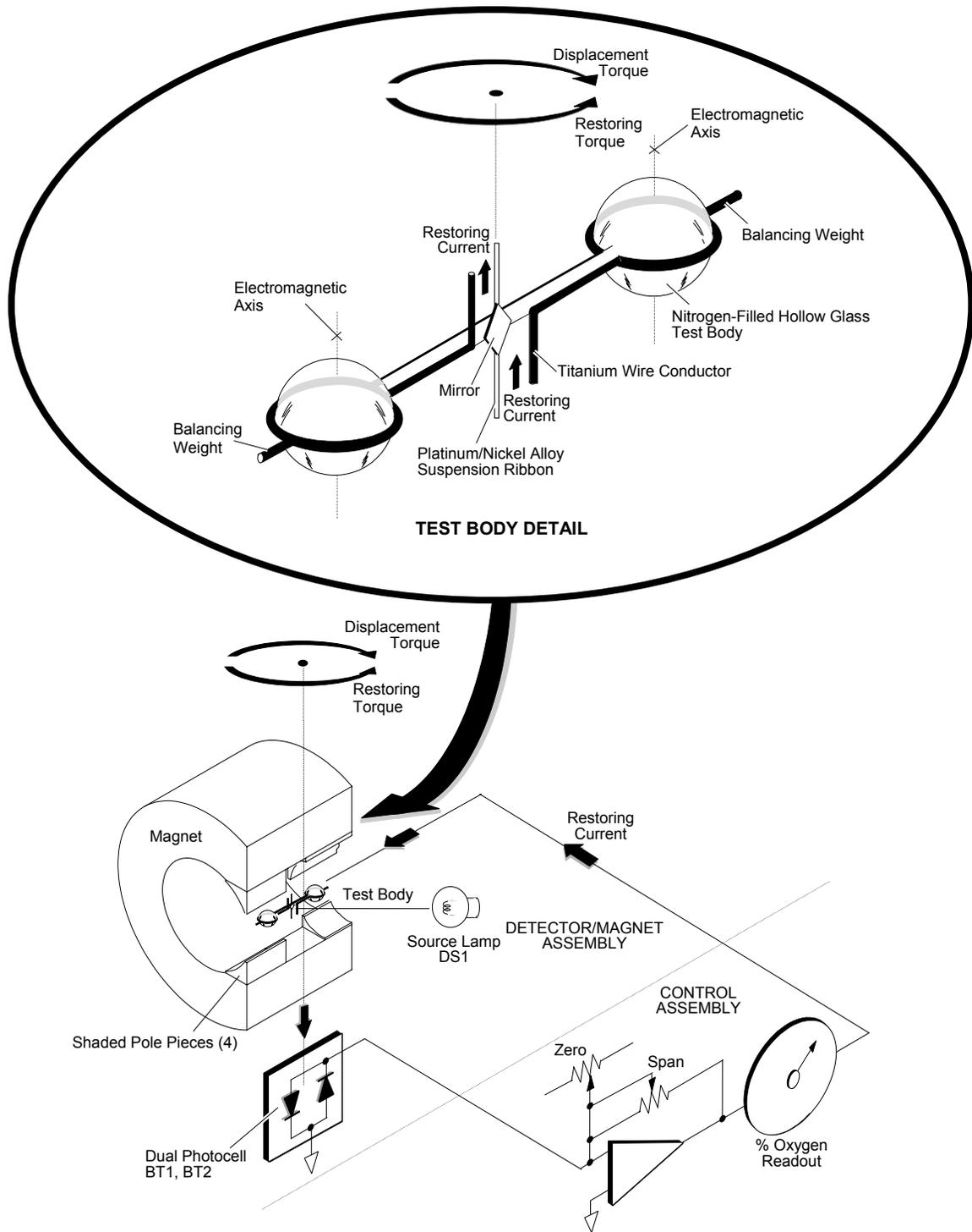
Figure 4-1. Functional Diagram of Paramagnetic Oxygen Measurement System
