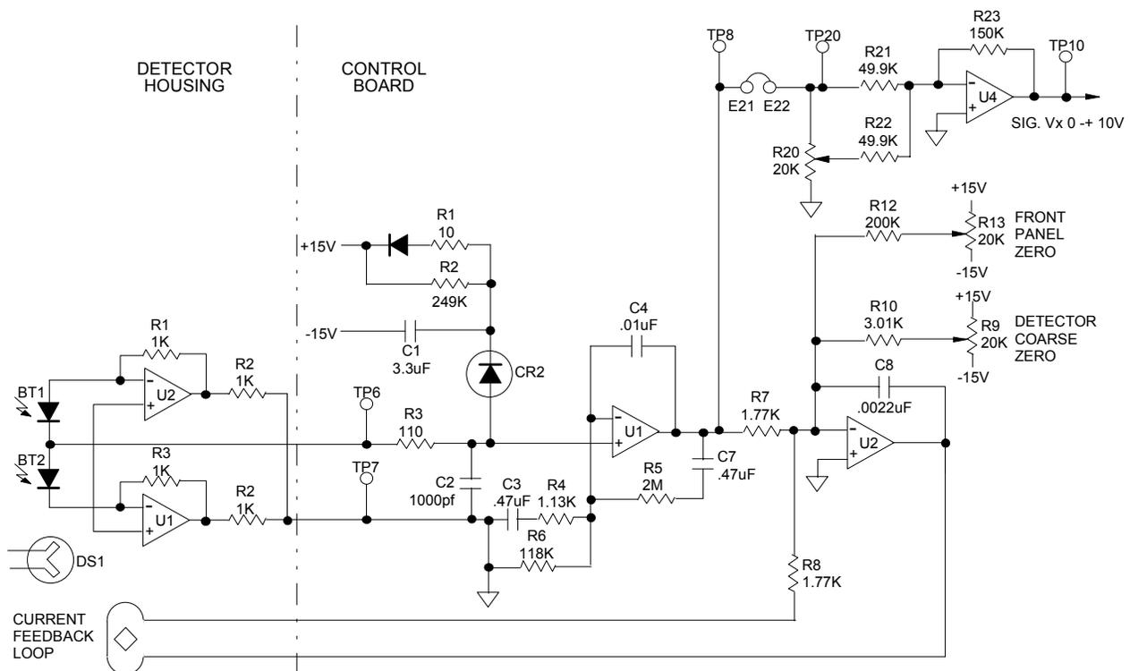
**Figure 5-6. Detector with First Stage Amplifier**
