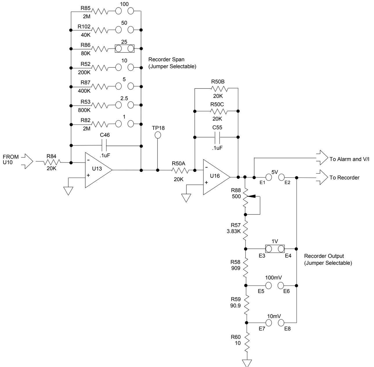
Figure 5-8. Simplified Analog Recorder Output Circuit
