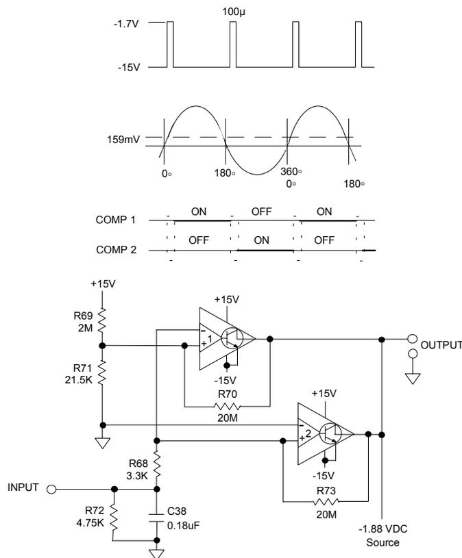
Figure 5-1. Two-Comparator OR Circuit
