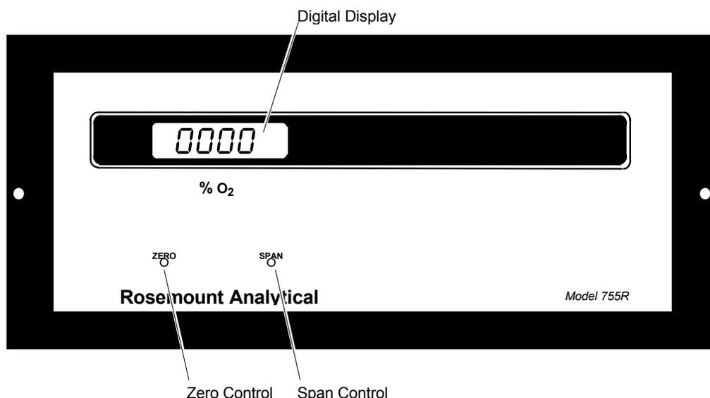
**Figure 1-1. Model 755R Oxygen Analyzer – Front Panel**
