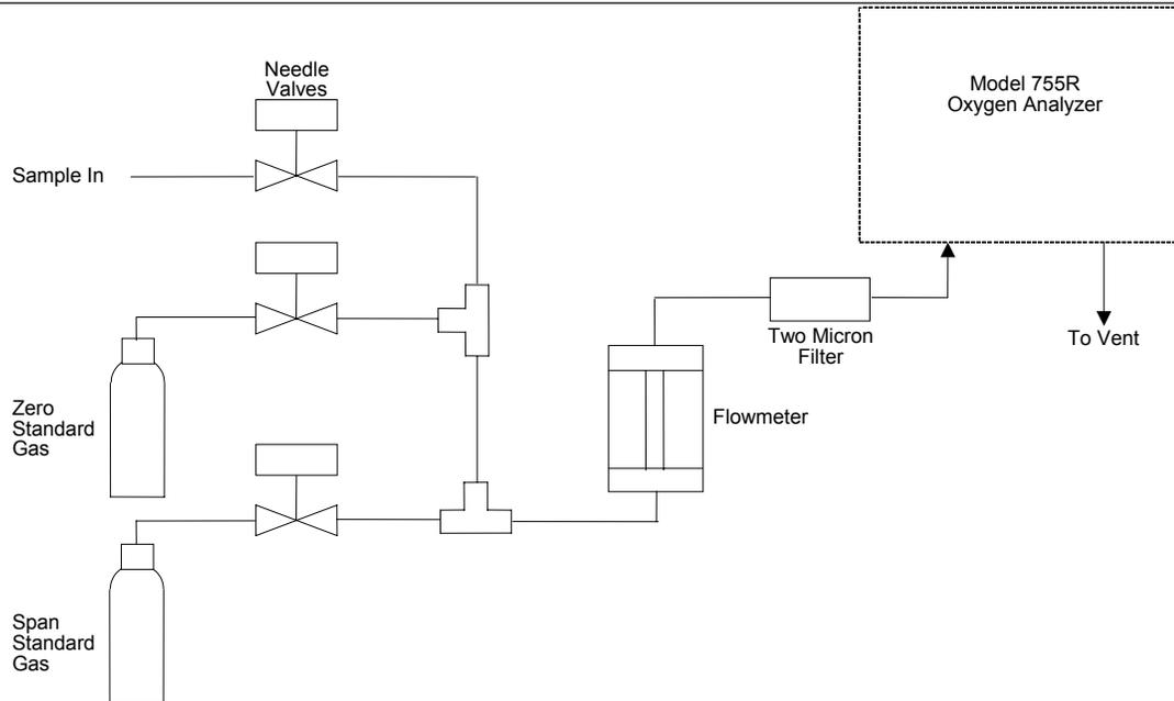
**Figure 2-1. Interconnect of Typical Gas Manifold to Model 755R**
