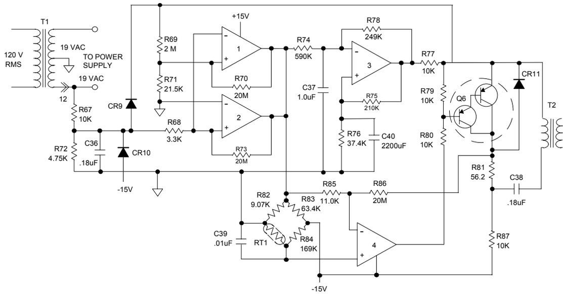
Figure 5-2. Case Heater Control Circuit
