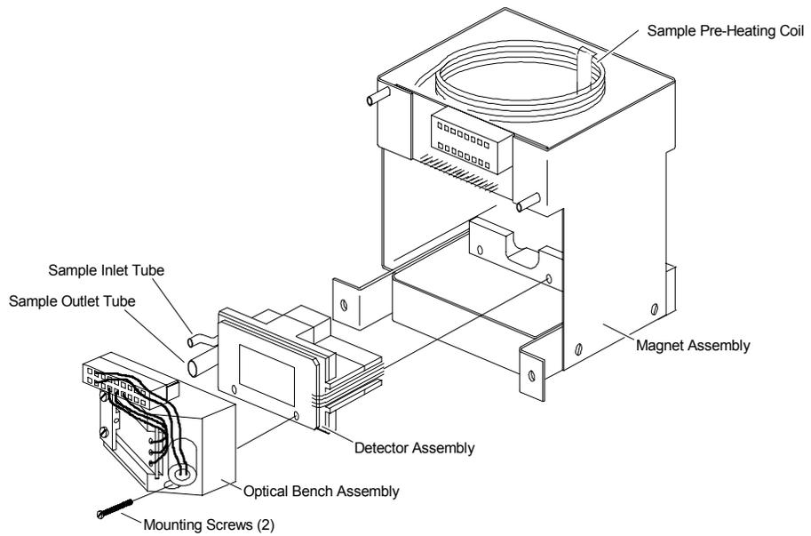
A. Exploded View of Detector/Magnet Assembly
