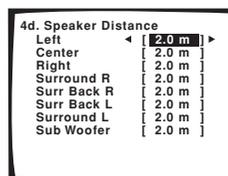
You can adjust the distance of each speaker in 0.1 meter increments.
