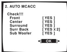
If the speaker configuration displayed isn't correct, use the **↑/↓** (cursor up/down) buttons to select the speaker and **←/→** (cursor left/right) to change the setting (and number for surround back). When you're finished, go to the next step.
