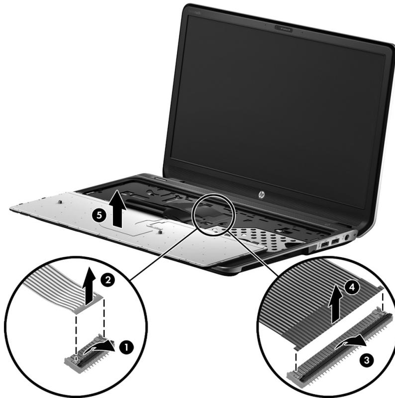
Reverse this procedure to install the keyboard.
