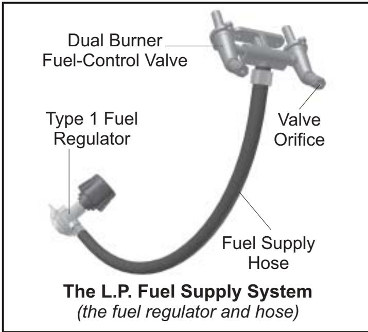
4. The pressure regulator and hose assembly provided is factory set at an outlet pressure of 11 inches water column (.4 lb. per sq. Inch).
