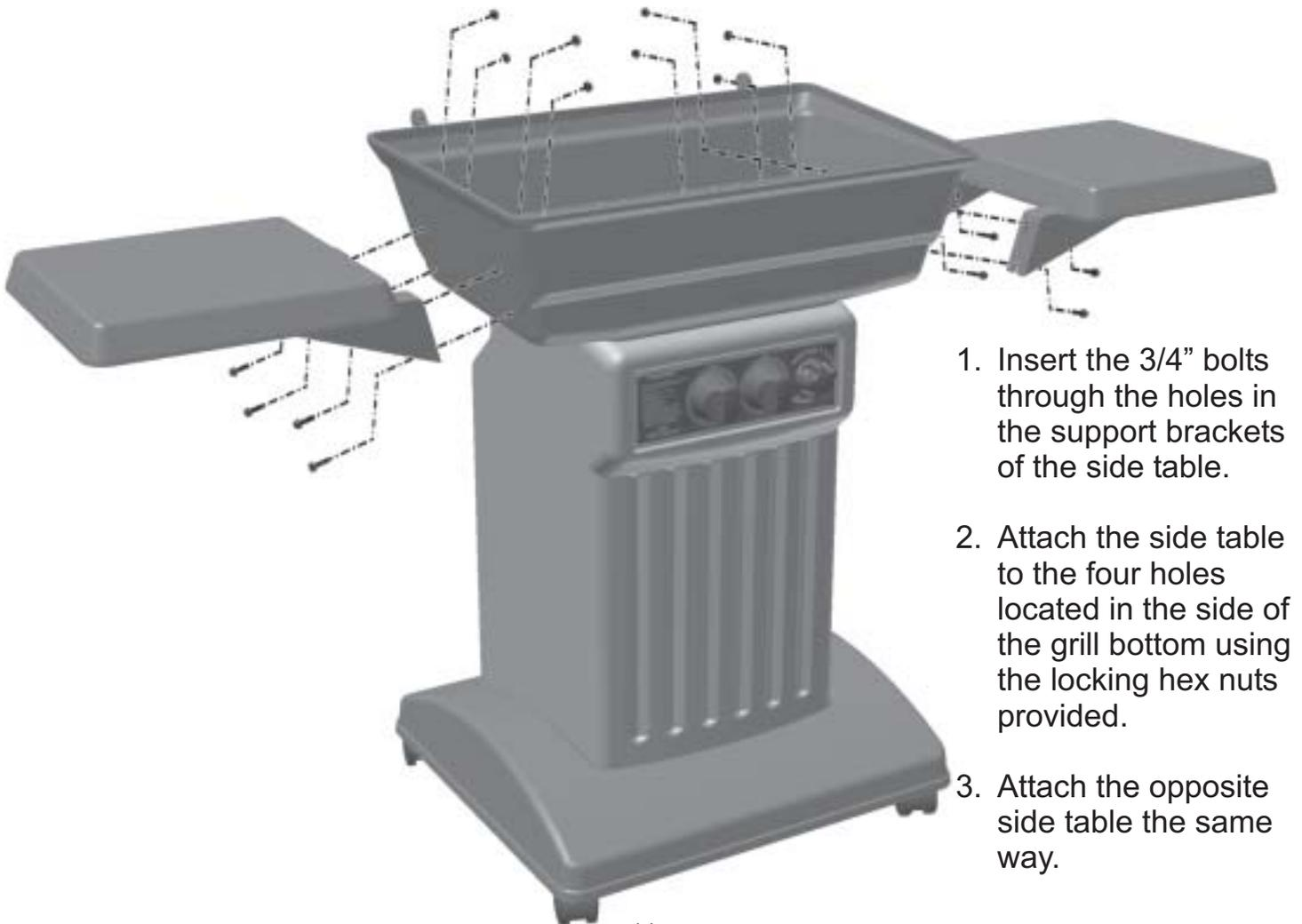
1. Insert the 3/4" bolts through the holes in the support brackets of the side table.
