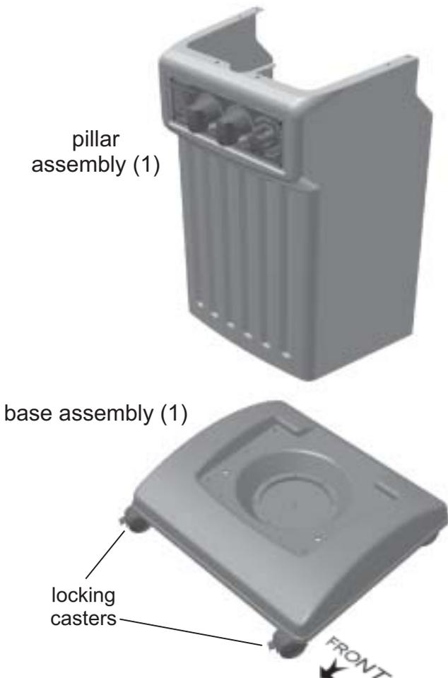
1. Lock the pre-assembled casters on base by pushing down on the latch.
