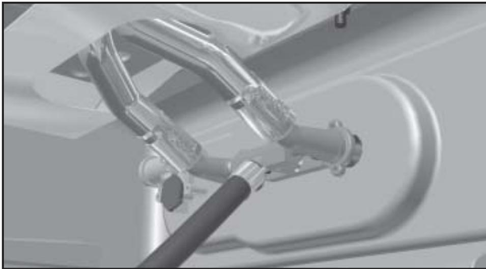
Improper installation and connection of the burner tubes to the control valves is dangerous and may lead to damaging fire and personal injury.
