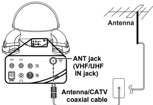
1. Connect one end of the VHF/UHF (Antenna) or CATV cable to ANT Jack (VHF/UHF IN Jack) on the back of the TV.
