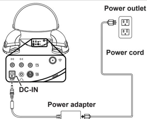
1. Connect the power cord to the power adapter as illustrated.
