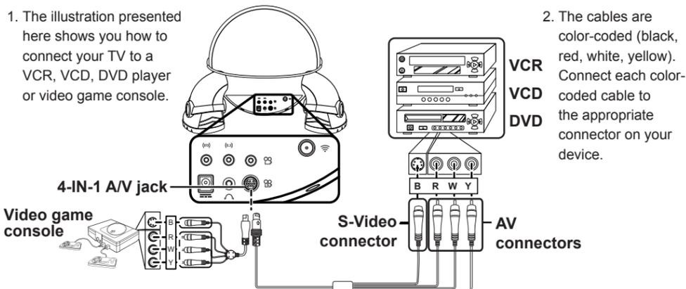
2. The cables are color-coded (black, red, white, yellow). Connect each color-coded cable to the appropriate connector on your device.
