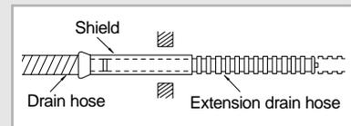
➤ **The hose will be fixed permanently into position once the whole installation has been tested for gas leaks; refer to page 46 for further details.**
