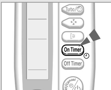
1 To set the operating time, press the ON TIMER button one or more times until the required time is displayed. Possible time is between 0.5 hour and 24 hour inclusive.
