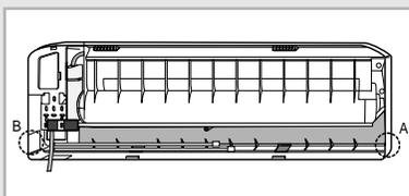
1 With a knife, cut out the appropriate knock-out piece on the rear of the indoor unit (unless you are connecting directly from the rear).
