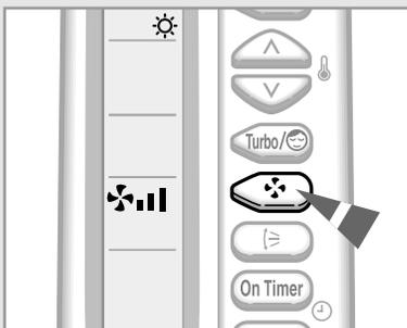
4 Select the fan speed by pressing the FAN button one or more times until the required setting is displayed:
