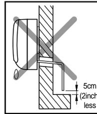
Keep a clearance of at least 5cm(2inch) between the end of the hose and the ground.
