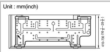
**1** Determine the position of the pipe and drain hose hole using the right figure and drill the hole with an inner diameter of 65mm (2 <sup>9</sup>/<sub>16</sub> inch) so that it slants slightly downwards.
