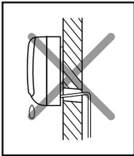
The hose must NOT slope upwards.
