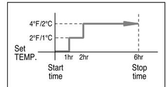
**Heating** The desired temperature is decreased by 2°F/1°C every hour. When it has been decreased by 4°F/2°C (after two hours), the temperature is maintained for four hours.
