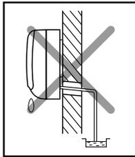
The end of the drain hose must NOT be placed in water.
