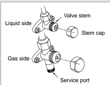
**1** Connect each assembly pipe to the appropriate valve on the outdoor unit and tighten the flare nut.
