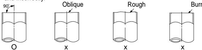
3 To prevent any gas from leaking out, remove all burrs at the cut end of the pipe, using a reamer.
