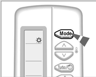
2 If the
