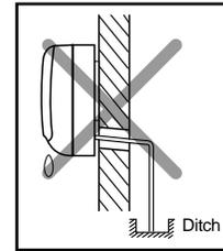
Do NOT place the end of the drain hose in a hollow.
