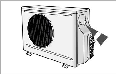
**One electric cable must be connected to the outdoor unit:**
