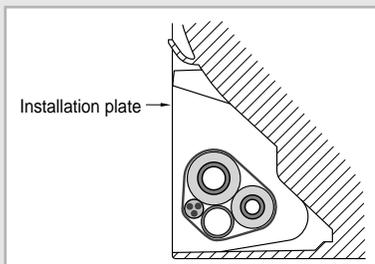
**Once you have checked that there are no leaks in the system, you can insulate the piping, hose and cables and place the indoor unit on the installation plate.**
