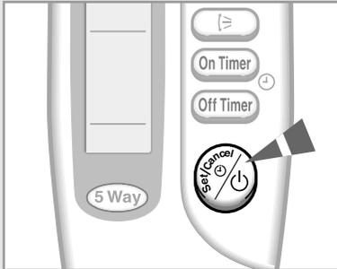
1 If necessary, press the
