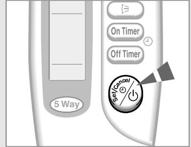
2 If the
