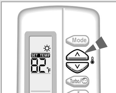
3 To adjust the temperature, press the TEMPERATURE buttons one or more times until the required temperature is displayed.
