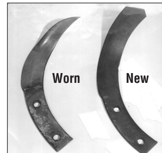
Figure 5-30: Check for wear every 30 operating hours.
