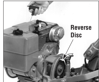
Figure 5-25: Checking Reverse Disc in NEUTRAL.
