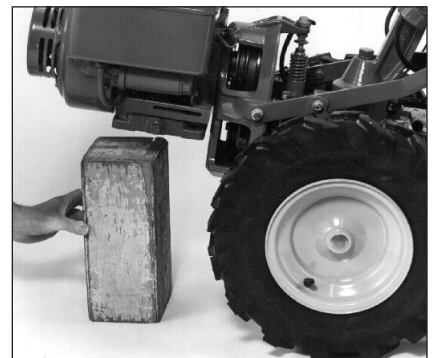
Figure 4-23: Block up engine.
