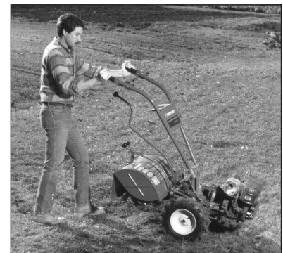
Figure 4-5: Turning the tiller.
