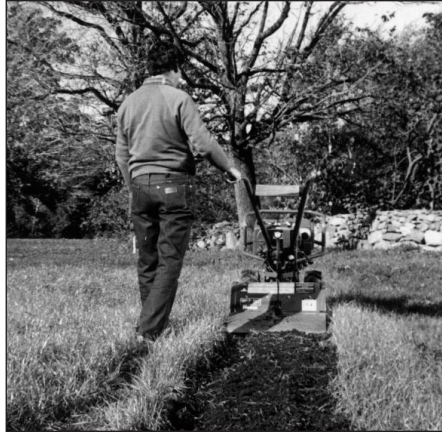
Figure 4-4: Guide tiller with one hand.
