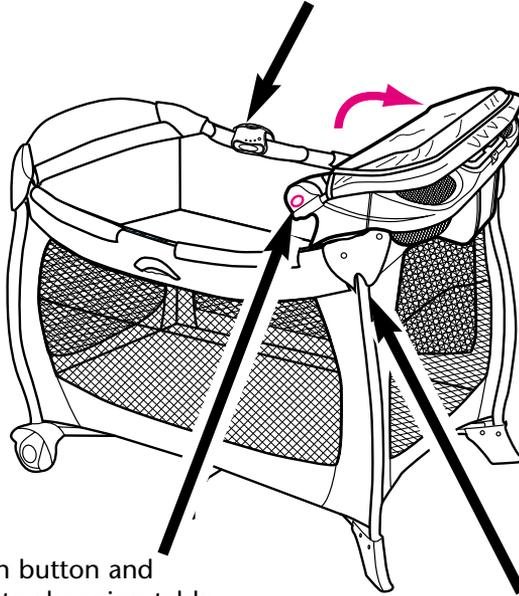
Push button and rotate changing table out of the way when not in use.
