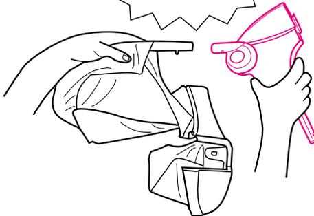
Snap tube into swivel mount on both sides.
