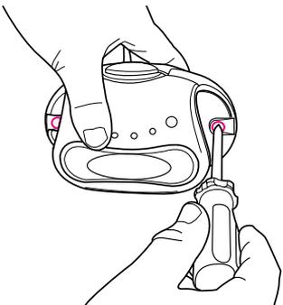
Remove 2 screws from back of electronics module.
