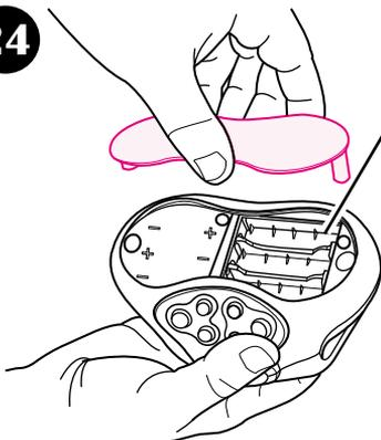
Remove battery door and insert 3 "AA-LR6" batteries. Replace door and screws.
