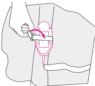
Vibrator must be fastened tight and centered on the webbing strap to work properly.
