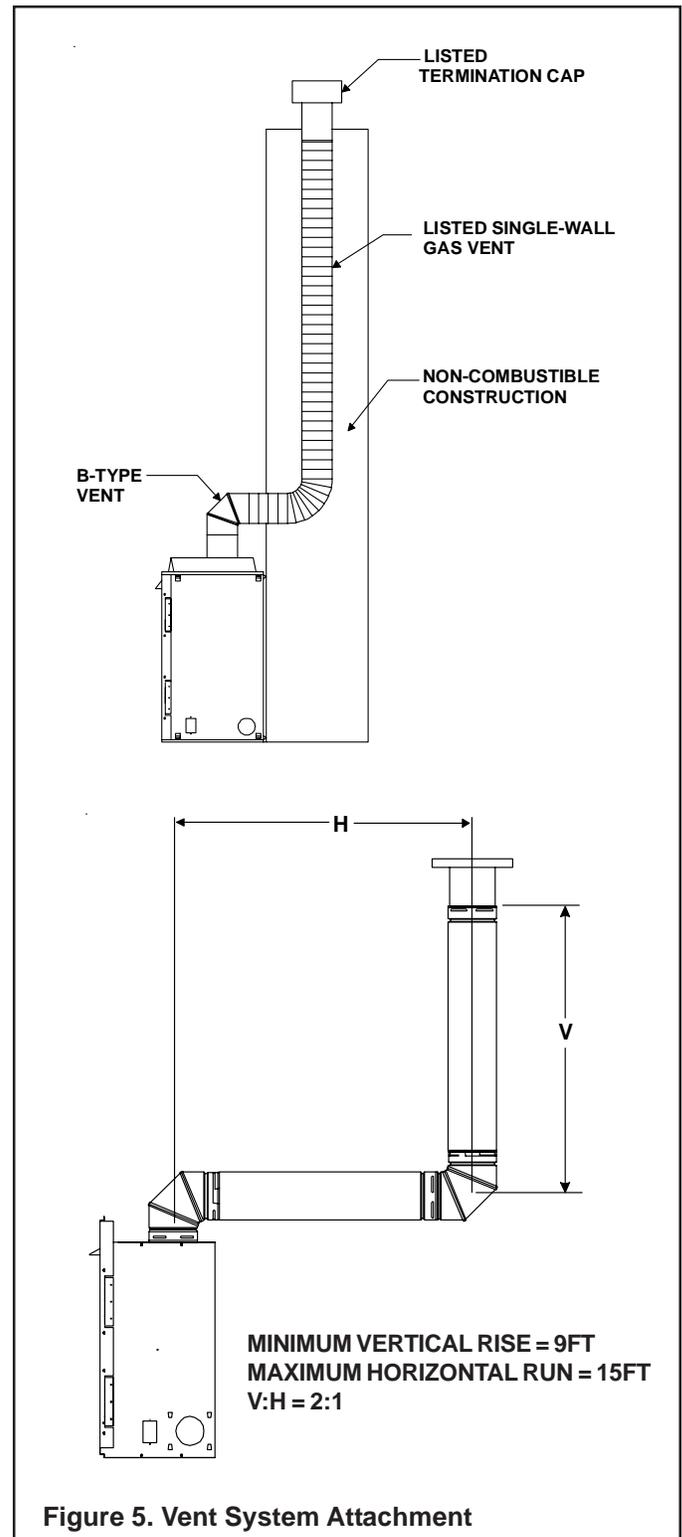
Figure 5. Vent System Attachment
