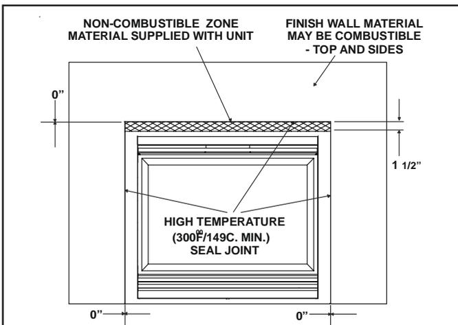
**Figure 14.** Sealant Material
