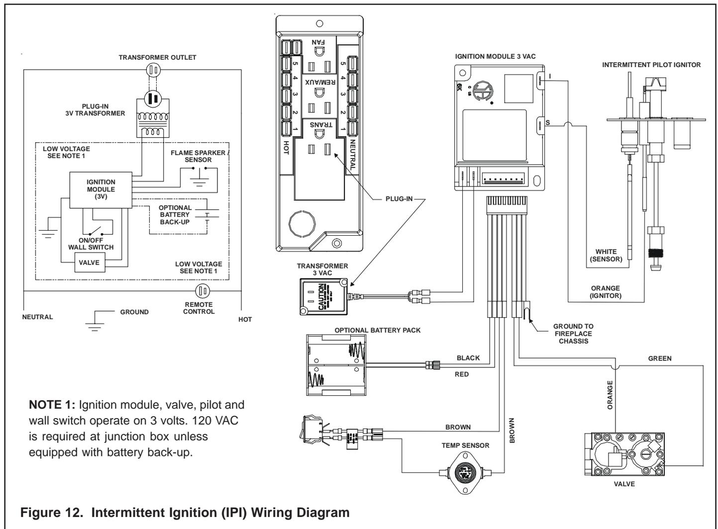
Figure 12. Intermittent Ignition (IPI) Wiring Diagram
