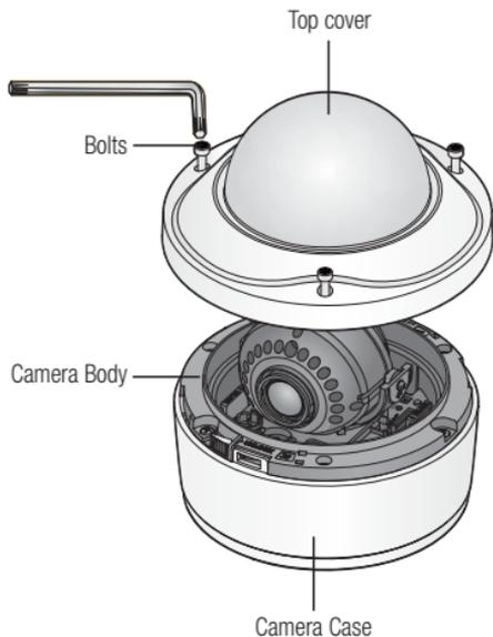
2. Loosen 3 screws on the camera body counter clockwise, and push down the left/right LOCKER lever (in the arrow direction) to release the lock. Then, remove the camera from the case.
