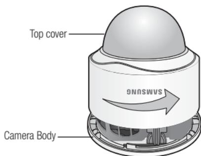
2. Press the <UNLOCK> levers on both ends to separate camera module from the body.
