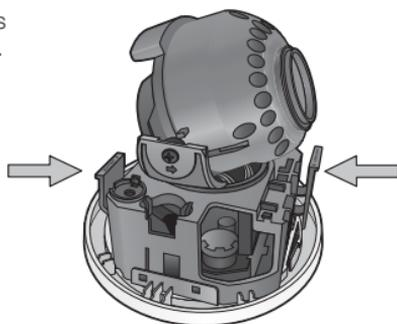
3. Hold down the lock lever in the outer direction as shown and turn the camera body in the <UNLOCK> direction (counter clockwise) to remove the bracket from the body.
