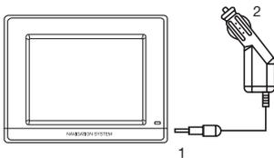
When the battery is in a low voltage, you can recharge it in the car:
