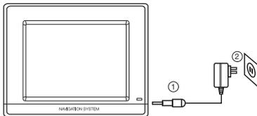
Push the adapter connector into the guide on the right of the network adapter. Push the Network Adapter (2) into a power point that is easily accessible.
