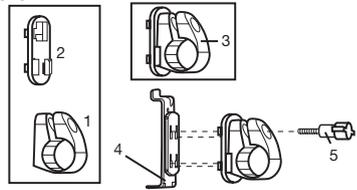
1. Place the clip (1) and the Retaining Plate (2) together and fix them to your bicycle handlebars by pulling them across the handlebars from below and pushing one of the rubber rings (3) supplied between the clip and the handlebars. The flat site of the support points in your direction. As the material is elastic, you can care fully bend open the support, lay it around the handlebar and push it together again.
