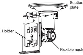
3. Mount the car holder to the flexible neck. Note the labels on the flexible neck. The arrow labeled **CLOSE** must point in the direction of the fixture. The connection closes with a noticeable clicking sound.
