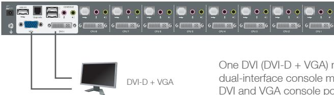
One DVI (DVI-D + VGA) monitor – plug your dual-interface console monitor into both the DVI and VGA console ports
