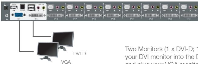
Two Monitors (1 x DVI-D; 1 x VGA) – plug your DVI monitor into the DVI console port, and plug your VGA monitor into the VGA console port.
