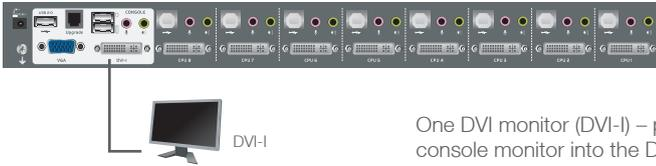
One DVI monitor (DVI-I) – plug your DVI console monitor into the DVI console port located on the unit's rear panel;
