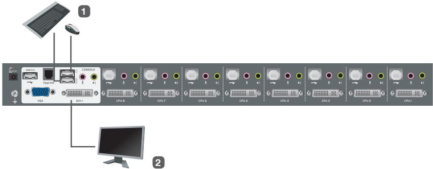
2. Depending on your console monitor's interface, connect your monitor using one of the following methods (**see Console Monitor Connection Options, page 8**), and power on:
