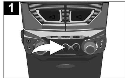
1 Rotate the ECHO control clockwise to increase the echo or counterclockwise to decrease the echo.
