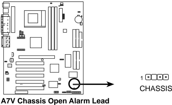
A7V Chassis Open Alarm Lead
