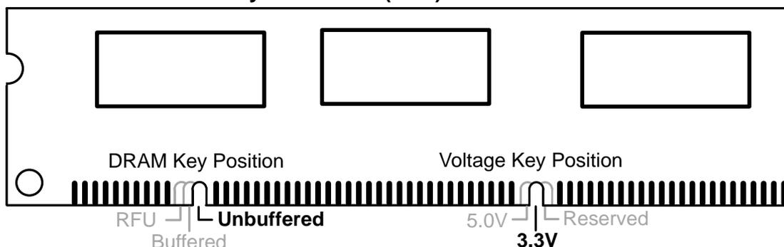
The notches on the DIMM will shift between left, center, or right to identify the type and also to prevent the wrong type from being inserted into the DIMM slot on the motherboard. You must tell your retailer the correct DIMM type before purchasing. This motherboard supports four clock signals per DIMM.
