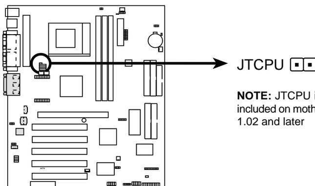
**NOTE:** JTCPU is no longer necessary/not included on motherboards with PCB versions 1.02 and later
