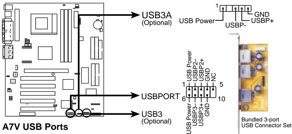
**Recommended Setup:** Use USBPORT + USB3A with the bundled 3-port connector set.
