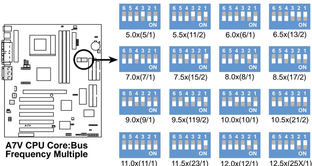
**NOTE:** If your processor does not have a locked Frequency Multiple, you must use **CPU Core:Bus Freq. Multiple** to set the Frequency Multiple. If the Frequency Multiple of your processor is locked, setting the Frequency Multiple will have no effect.
