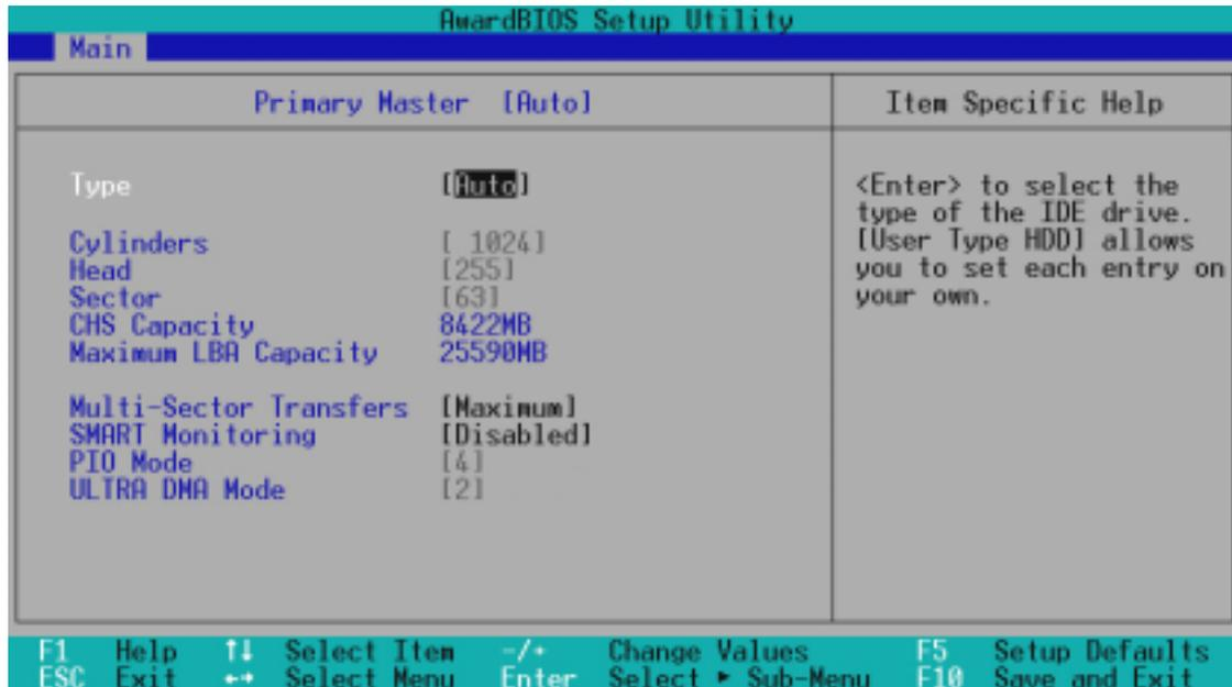
**NOTE:** Before attempting to configure a hard disk drive, make sure you have the configuration information supplied by the manufacturer of the drive. Incorrect settings may cause your system to not recognize the installed hard disk. To allow the BIOS to detect the drive type automatically, select [Auto].
