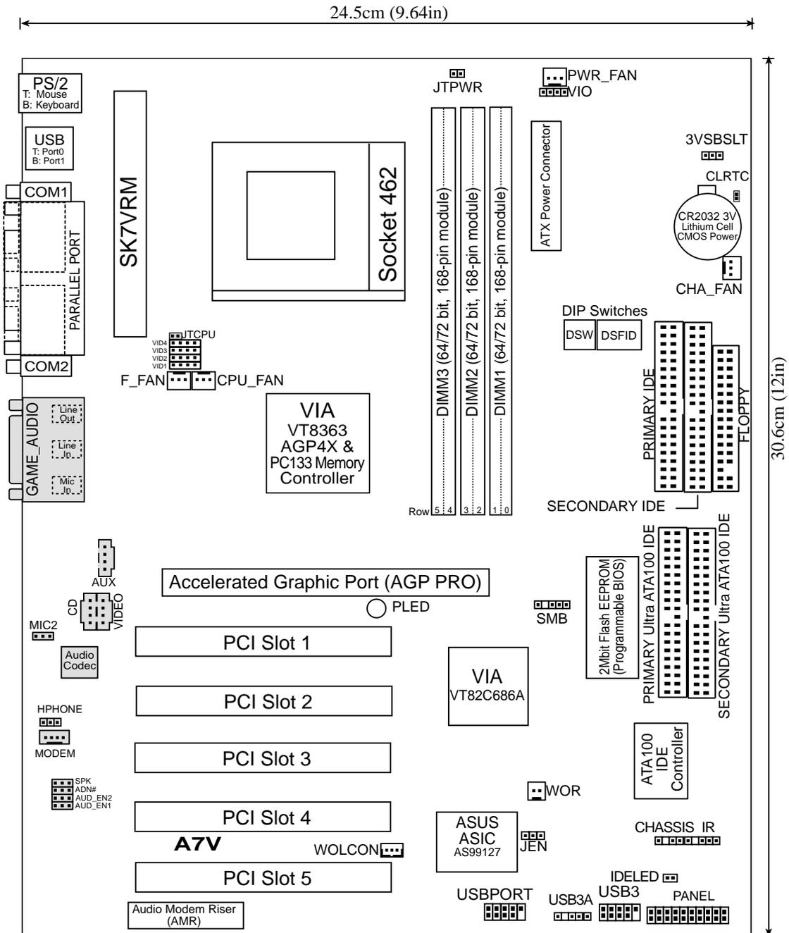
Grayed components are optional at the time of purchase (JTCPU is no longer necessary on motherboards with PCB versions 1.02 and later)
