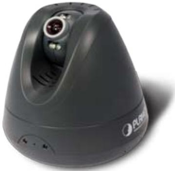
The PLANET ICA-M230, built-in high performance 1.3Mega-Pixel CMOS sensor delivers high quality image at maximum 1280x1024 resolution, multi-profile stands for video stream simultaneously. The ICA-M230 can generate MPEG-4 and M-JPEG streaming to different users in the at the same time. Moreover, the resolution can differ from one user to another. This state-of-the-art design is considerably able to fit in various network environments. The ICA-M230 allows up to 10 users to access simultaneously.
