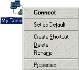
Picture 5. Changing connection properties (click right mouse button and choose P roperties).
