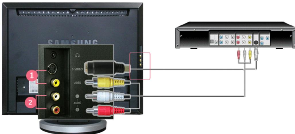
1. Input devices such as DVD, VCR or Camcorder are connected to the VIDEO or S-VIDEO terminal of the monitor using the Video or S-Video cable.
