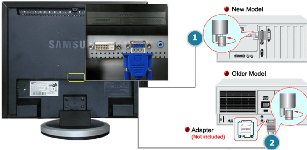
1. Using the D-sub (Analog) connector on the video card.
