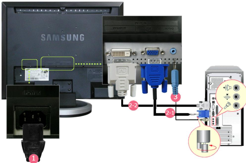
1. Connect the power cord for your monitor to the **POWER** on the back of the monitor. Plug the power cord for the monitor into a nearby outlet.
