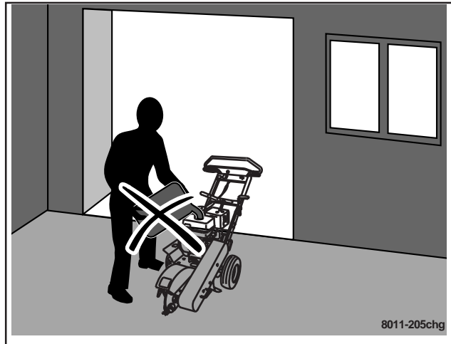
Never fill the fuel tank indoors.
