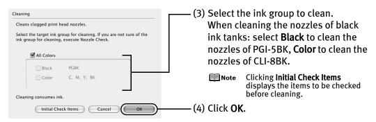
**Print Head Cleaning** starts when the **POWER** lamp starts blinking green.
