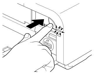
**▶** Important If the **ALARM** lamp begins flashing orange, refer to "**Handling Error Messages**" on page 77.
