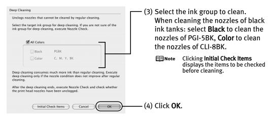
**Print Head Deep Cleaning** starts when the **POWER** lamp starts blinking green.
