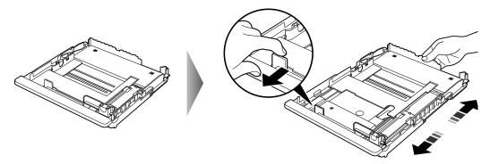
When loading  $5" \times 7"$ - or smaller sized paper (nonstandard-size paper: less than 203 mm/ 8 inches in length), do not extend the Cassette.
