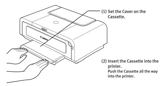
Note If the Cassette has been extended to accommodate paper sizes larger than 5" x 7", the front edge of the cassette will extend beyond the front of the printer.
