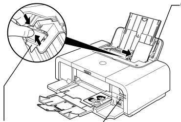
(2) Pinch the paper guide and slide it against the left side of the paper stack.
