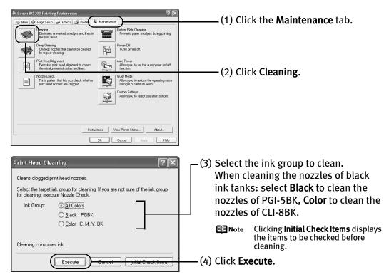
Print Head Cleaning starts when the POWER lamp starts blinking green.
