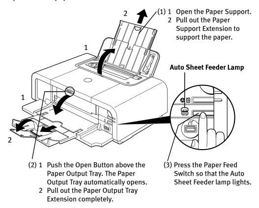
**Note** You can also select the paper source with the printer driver. For details, refer to the *Printer Driver Guide*.
