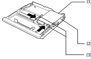
(1) Load the paper into the Cassette with the print side facing DOWN.
