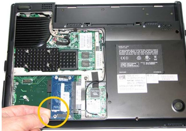
**Figure 8 Removing screws from newer-type flash module**
