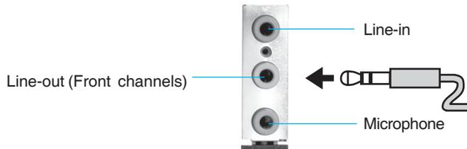
**Description:** Line-out, Line-in and Microphone functions all exist under 2-Channel configuration.
