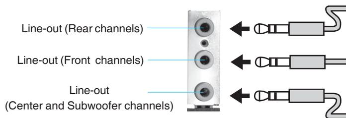
**Description:** Both Line-in and Microphone are converted to Line-out under the 6-channel configuration.
