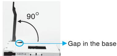
2. Align the cut edge to the gap in the base of the socket. Carefully insert the CPU into the socket until it fits in place.
