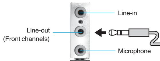
When using a 6-Channel sound source, connect the front speaker to the green audio output; connect the surround sound speaker to the blue audio input; connect the center speaker/subwoofer to the red Microphone input, as shown in the following figure:
