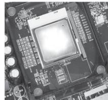
Note: The CPU heatsink may have a pre-applied thermal compound. In that case, the silica gel is not required.
