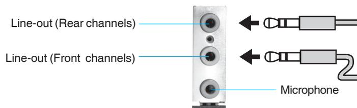
**Description:** Line-in is converted to Line-out under the 4-Channel configuration.
