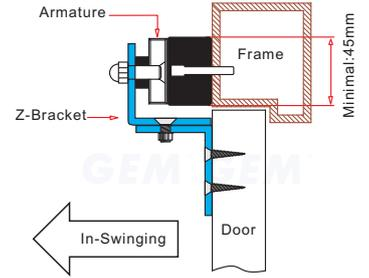
■ Application for the Electromagnet: GL-850
