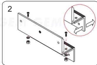
2 Assemble the Z bracket, and make sure that the Z bracket is adjustable.
