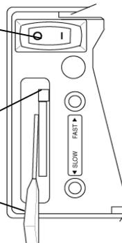
*Briggs Vanguard Units have an engine mounted throttle control.*
