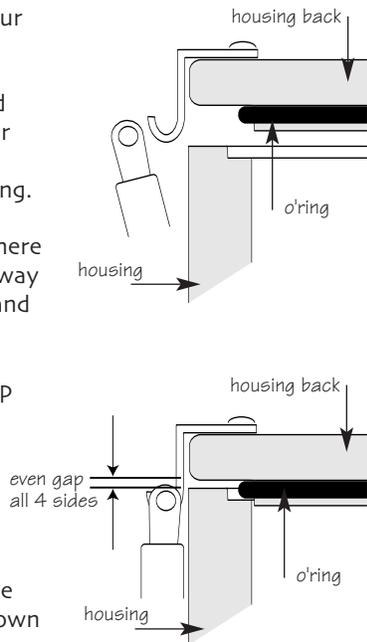
**Double check** - Once the housing is closed, check the o'ring seal.
