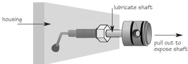
pulled out, exposing the shaft (see drawing).
