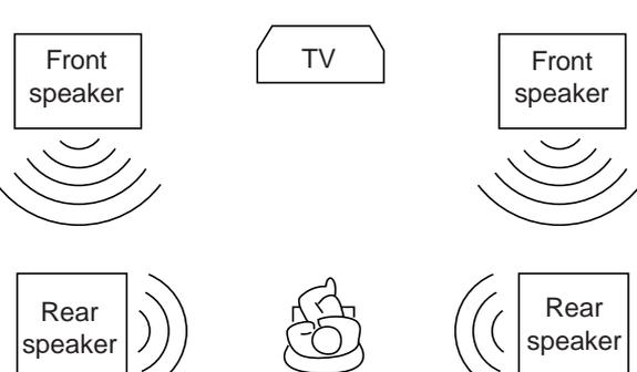
You can use Dolby Pro Logic in Center Phantom mode with this speaker configuration.
