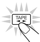
When the tape plays to the end, the deck automatically stops if the Reverse Mode is not on. (See “To play both sides repeatedly — Reverse Mode.”)
