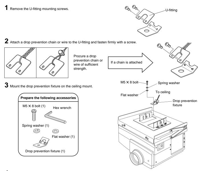
4 Attach the drop prevention fixture to the ceiling using the same procedure as described in items 1 - 3.
