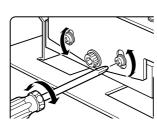
(5) Use the tilt adjustment screws (4 locations: 2 in front and 2 at the rear) to adjust the projector so that the projected image is not tilted in relation to the screen, then securely tighten the screws.
