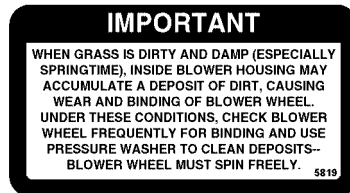
Top of Blower Housing (5819)
