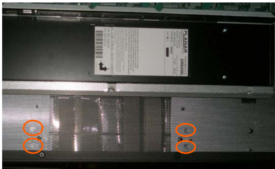
Landscape holes for kickstand bracket installation
